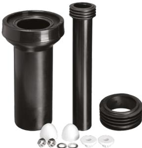
Kit comprises WC connector with 97-107mm Inlet, 4"/110mm outlet, flush pipe with finned seal connector and fixing bolts and caps. Suitable for in-wall WC frames
